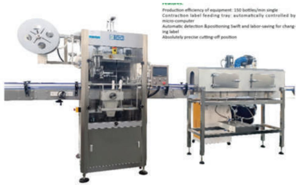
Production efficiency of equipment: 150 bottles/min single
